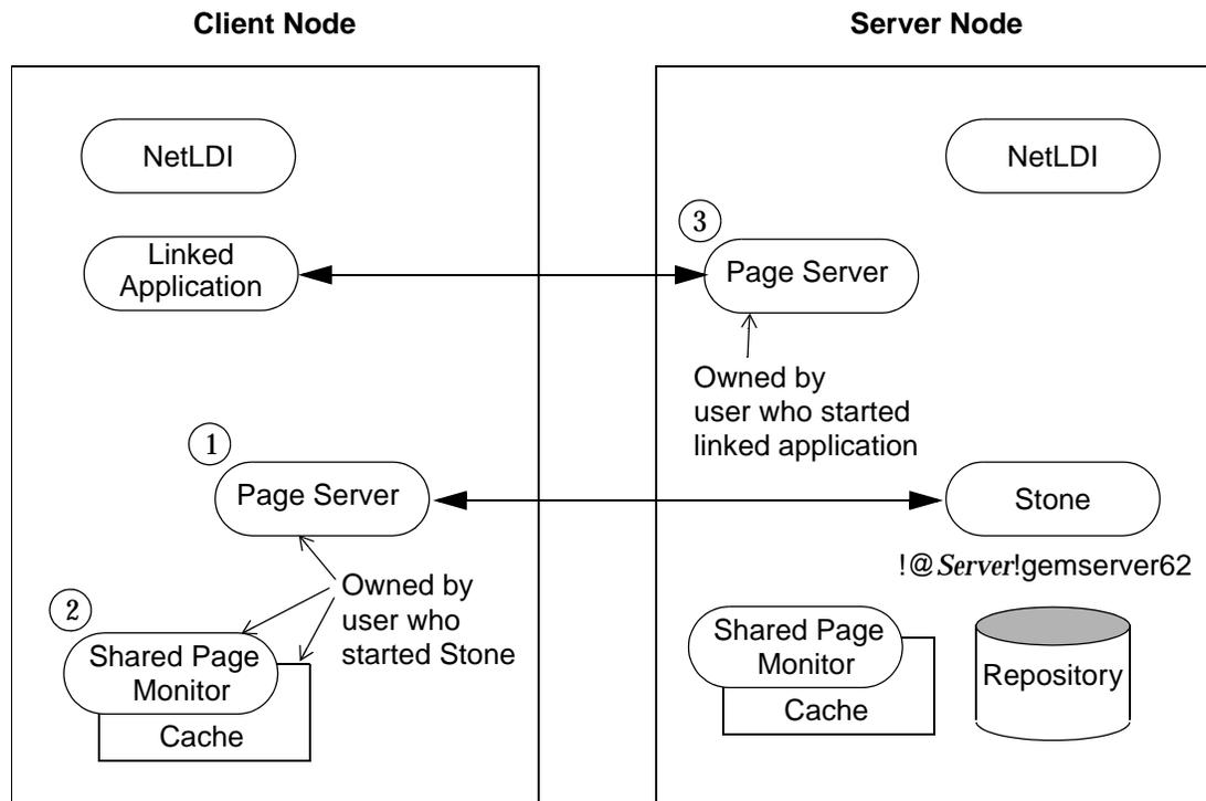
Two NetLDIs and two page servers ordinarily are required. NetLDIs start the page servers on request of the Stone and the application. Numbers show the order in which these processes are started:
