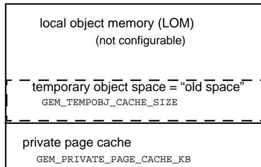
The Gem creates new objects smaller than 8 KB in local object memory, assigning each an object identifier. If the object is destined for persistence, it moves through local object memory generation by generation, at last ending in old space. Upon commit, the object is assigned a page in the private page cache and, from there, moves into the shared page cache.
