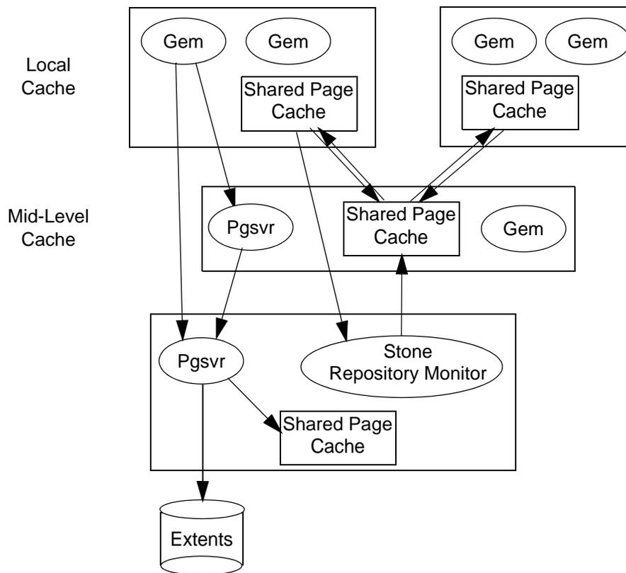
If a Gem is running on the same machine as a mid-level cache, that Gem will use the mid-level cache as its local cache.
