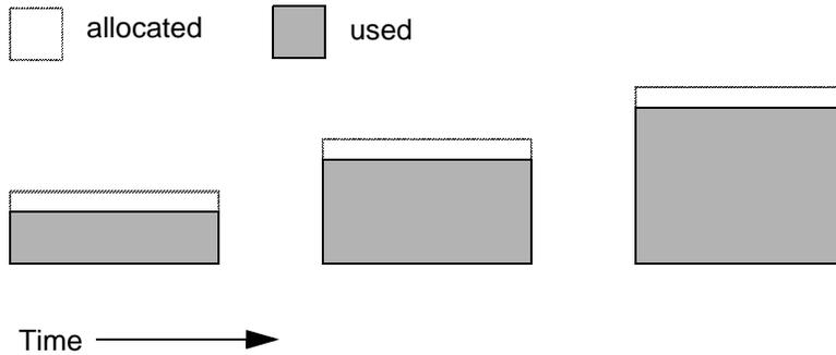
You can increase I/O efficiency while reducing file system fragmentation by instructing GemStone to allocate an extent to a predetermined size (called pregrowing it) at startup. When `DBF_PRE_GROW` is set to `True`, the Stone repository monitor obtains the necessary space when it creates a new extent or starts with an extent that is smaller than the specified size.
